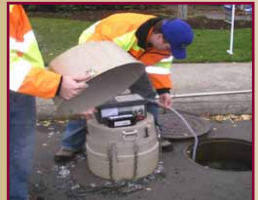
Inserting automated sampling equipment directly into a stormwater manhole.
