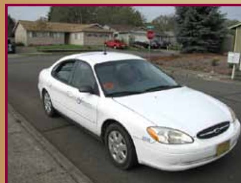
Meter reading vehicle equipped with radio reading technology (special antenna).
