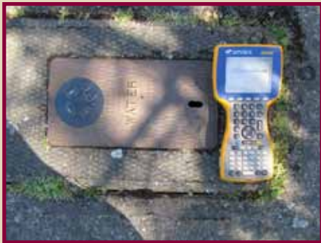
Handheld meter reading device and water meter lid.
