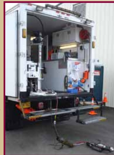
CCTV truck used for recording video inspections of new construction, pipe condition, and dye testing.
