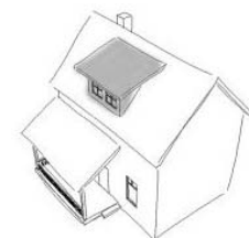
INCORRECT DORMER APPLICATION (ON FRONT OF STRUCTURE)
